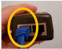
3. Take the other cord and insert one end into the Power Injector's POE port
